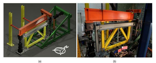
Figure 3. Layout of test setup: (a) AutoCAD rendering and (b) and as-built photo of setup.
